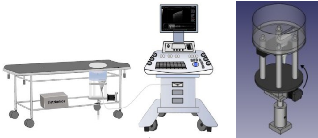
Figure 1: Illustration of the bed arrangement with the robot arm, a microcontroller, and a more detailed view of the robot arm. Adapted from [3].
